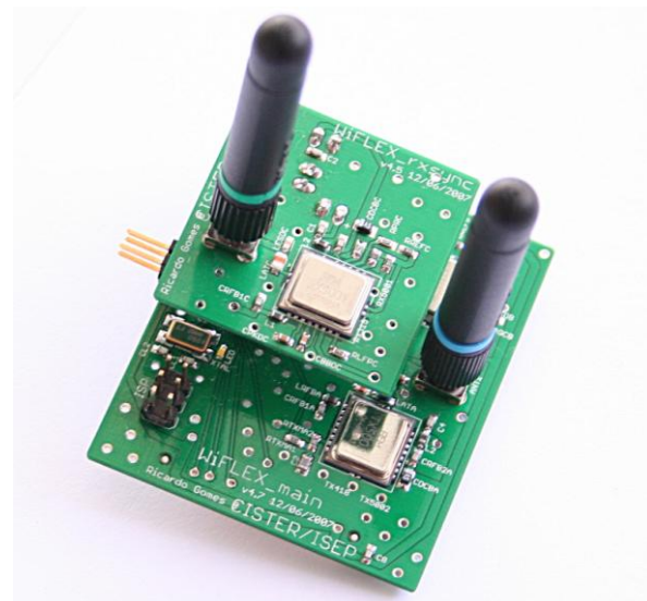
Prototype board for Dominance-based MAC protocols developed by CISTER
