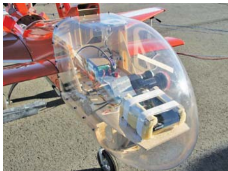
Figure 2 – The nose on the Brumby UAV houses the vision and IR sensors
